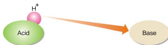
■ Figure 27.2 A Bronsted acid is a proton donor and a Bronsted base is a proton acceptor.
