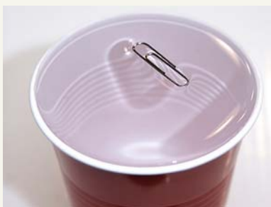
Surface tension prevents a paper clip from sinking.
