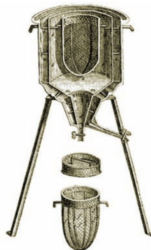
The world's first ice-calorimeter, used in the winter of 1782-83, by Antoine Lavoisier and Pierre-Simon Laplace, to determine the heat evolved in various chemical changes.
